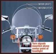
Available in two sizes and two styles for bikes with high or low turn signal placement.
