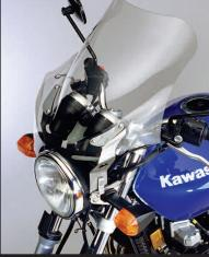
The F-15 is the original F-Series Fairing. The larger of the three styles is made from high impact acrylic. The fairing mounts to the motorcycle's headlight mount point using platinum colored aluminum uprights. The F-15 is the largest of the F-Series Fairings and is offered in two heights.
