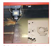
Engineered and precision laser cut, the stainless steel Paladin® and QuickSet™ components are durable and long lasting.
