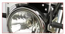
The Flyscreen for standard bikes uses Headlight-Mount hardware (included).
