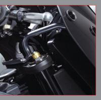
The one-piece B-King mounting system is attached between the risers and the top triple clamp for maximum strength. The black powdercoated finish matches the OEM hardware. Combined with a rubber grommet suspension to the screen, this VStream is an outstanding performer.
