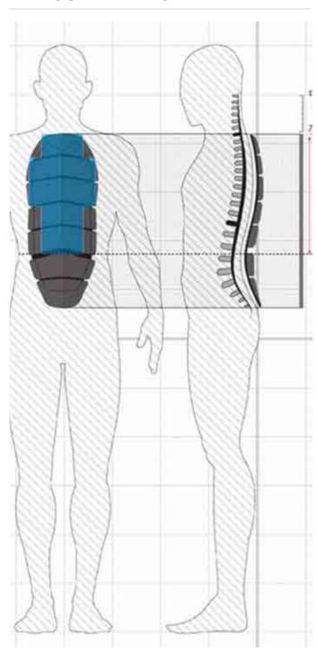
As it is not currently possible to industrially produce tailored back protectors, back protector must be worn by people with anthropometric characteristics lying within a certain range. A back protector is suitable for a person if its height does not exceed the seventh cervical vertebra and if the minimum area of the model is related to a waste shoulder height greater than or equal to that of the person.
