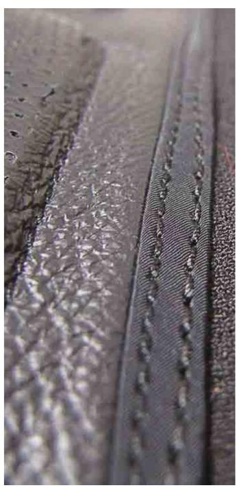
Each and every detail has a precise function: the pursuit of safety also demands careful study into the correct positioning of the stitching to both ensure greater comfort and prevent breakage that would remove protection and subject the wearer to greater risk during a spill.
