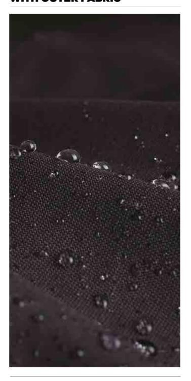
The fabric is laminated directly to the membrane and provided with heat-sealed internal seams. In addition to ensuring the characteristics of breathability and a waterproof, windproof seal, this construction significantly reduces the item's weight while preventing the body from absorbing rain, lowers the wind- chill effect, and promotes rapid drying.
