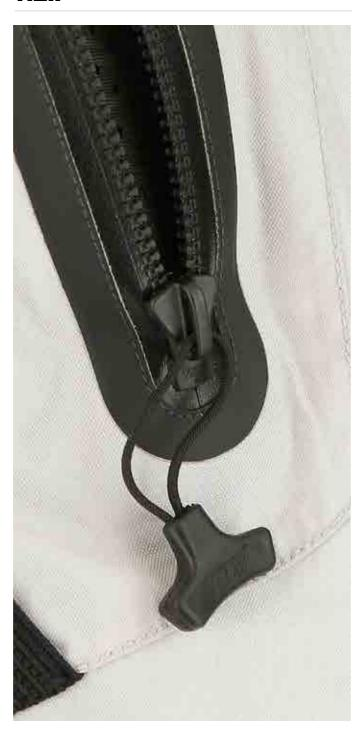
The TIZIP® MasterSeal is made from high-strength fabric coated with thermoplastic polyurethane. The extra strong plastic teeth are fixed on the top and bottom of the zipper tape. The zipper's coupling elements keep the sealing edges tightly sealed together when the zipper is closed. The zipper tape can be both welded and glued.
