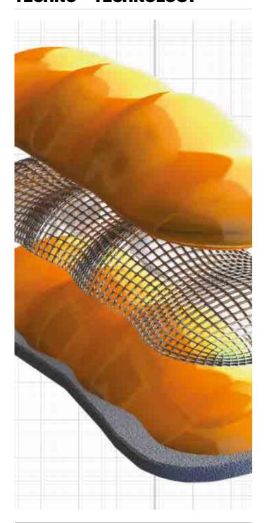
This exclusive patented Dainese technology used for the stiff inserts in gloves consists in the hot application of thermoformed inserts and a stainless steel net inside the fabric without stitching or layering that might otherwise weaken the glove's structure.
