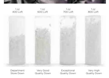
Fill Power is the volume-to-weight ratio of goose down filling that provides a clear indicator of product quality. The loftier the individual plumes are, the fewer are needed to obtain the desired volume. Consequently, the higher the Fill Power, the higher the quality of the down: high volume, low weight. Inside the Antartica Gore-Tex jacket is a 700 Fill Power jacket that provides this motorcycle garment exceptional insulation in conjunction with the highest degree of lightness.
