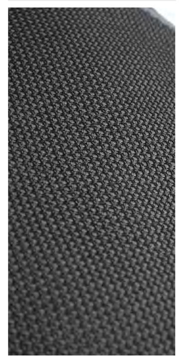
An innovative high-tech fabric, Dainese 3D Stone is constructed from 100% high-tenacity nylon in a special chunky three-dimensional weave that creates micro air-pockets. These retard abrasion for outstanding mechanical strength, which a polyurethane resin finish takes to even higher levels, achieving abrasion resistance of up to 8 seconds when tested to EN 13595-2
