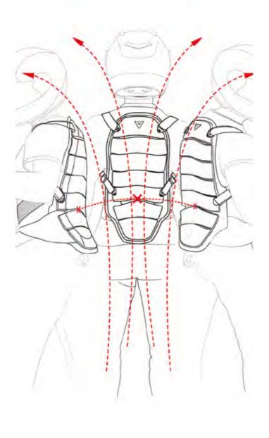
Active safety also means preventing accidents: the study of ergonomics underlies all Dainese\* protectors developed to follow the lines of the human body in order to ensure the greatest freedom of movement and increase comfort for the greatest concentration of attention on riding. One example is provided by the back protector developed with a sectional structure in order to permit both the total backward and forward bending of the trunk and lateral flexure thanks to the lumbar joint.
